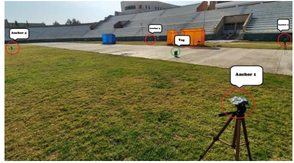
Fig. 9. LOS condition positioning environment.
