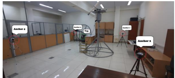
Fig. 10. NLOS condition positioning environment.
